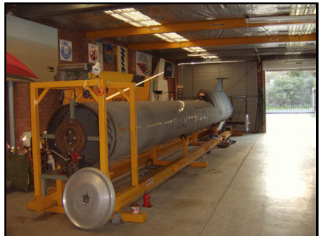
Front view of the cars mainframe on the purpose built jig
