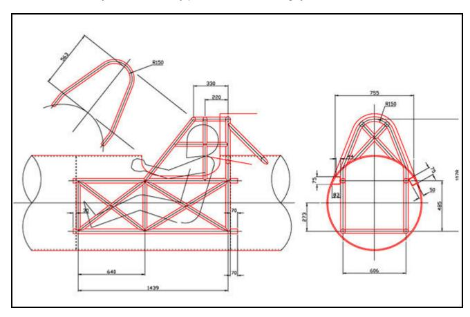
Mike, Terry and Kim all made suggestions on how this should be constructed and we believe we arrived at the perfect solution. This cage has to be made and fitted in 3 different sections, a bit like a jigsaw; hopefully they will have this built very soon. You can read about this in more detail on our website <a href="https://www.aussieinvader.com">www.aussieinvader.com</a>.
