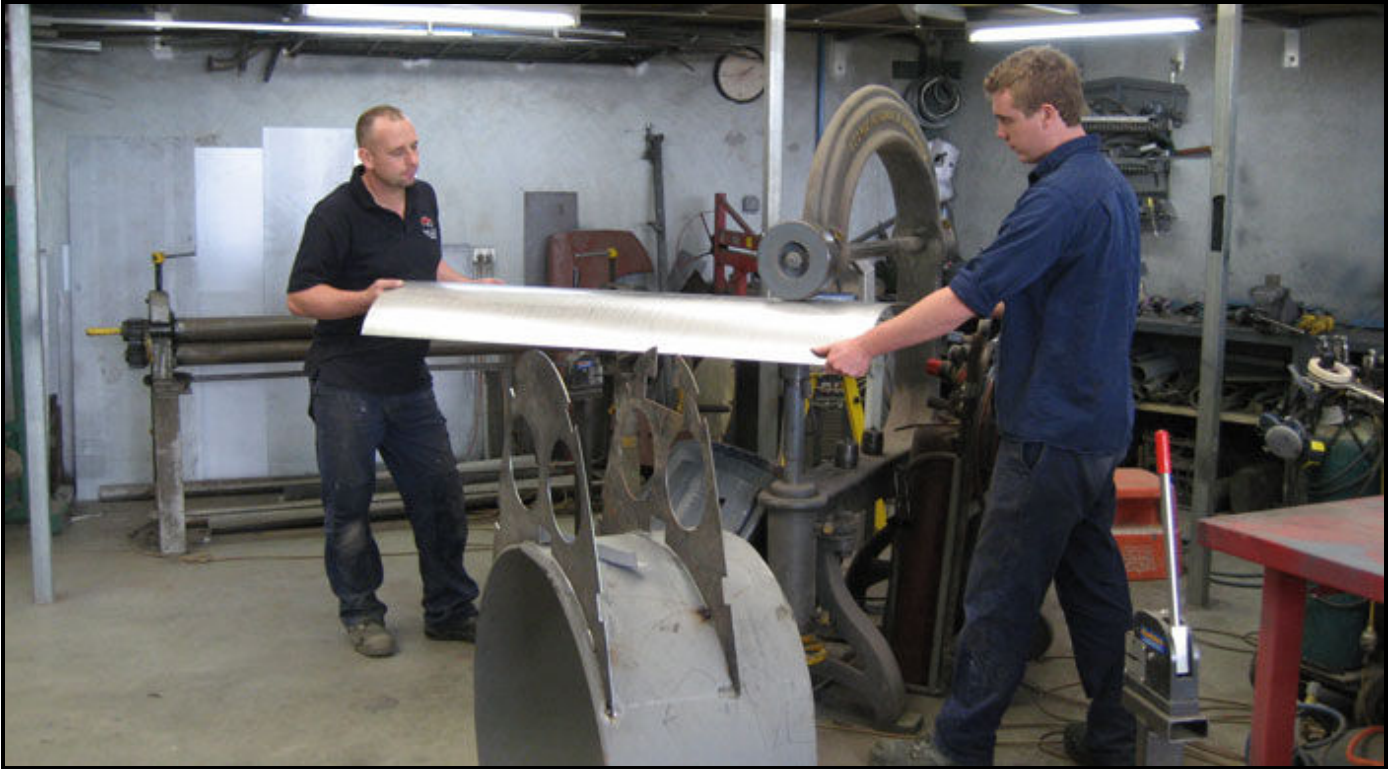
The guys at Rowe and Sons rolling our T3 sheets for our top-hat section
