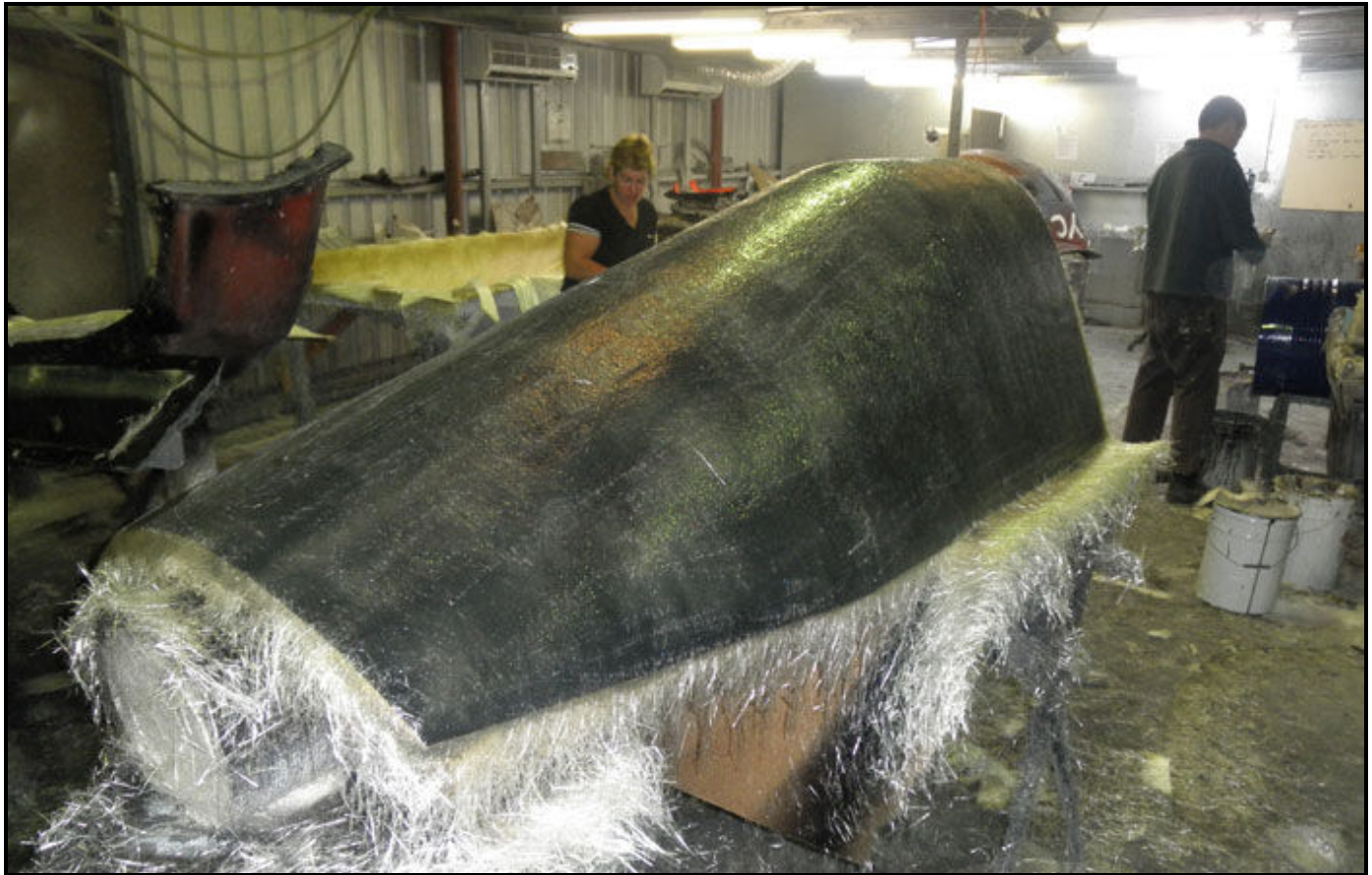
The canopy mould curing before separation
