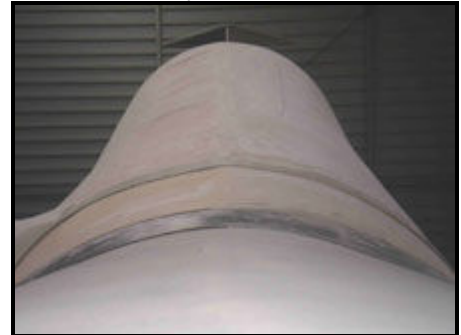
6. Canopy plug ready for moulding
