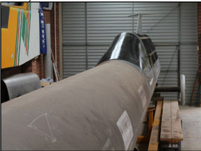
Canopy in place waiting for a meeting with a diamond bladed saw to cut the windshield area out and final fitting
