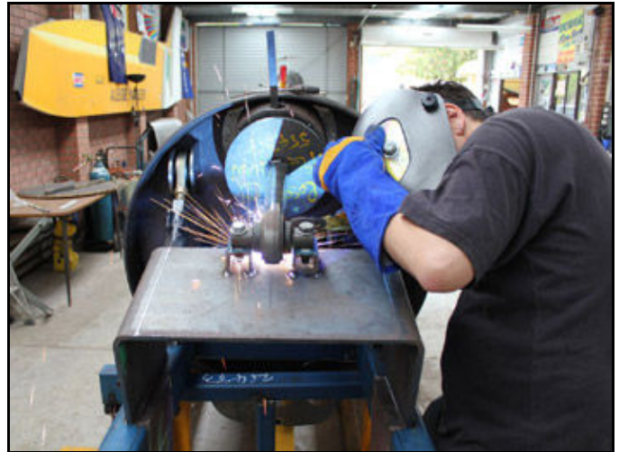
Alex welding the front suspensions main supports
