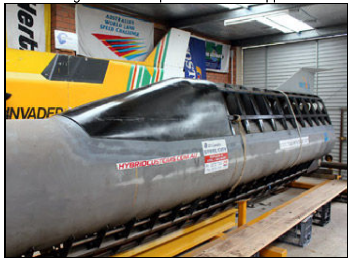
Canopy in place waiting for a meeting with a diamond bladed saw to cut the windshield area out and final fitting
