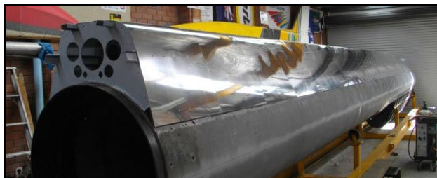
All panels in place before turning over
