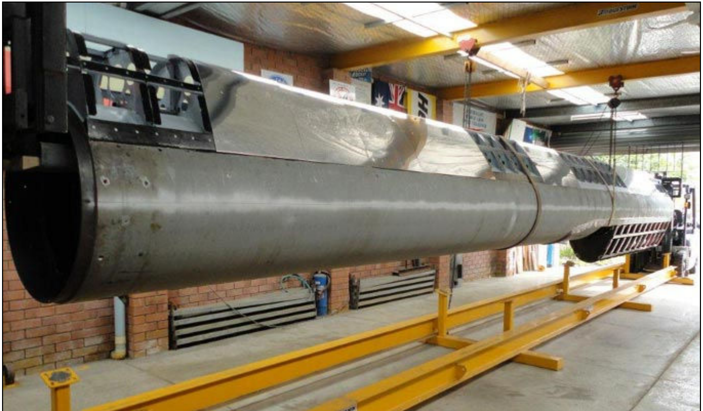
Tricky manoeuvre, turning the car over and removing the chassis jig.
