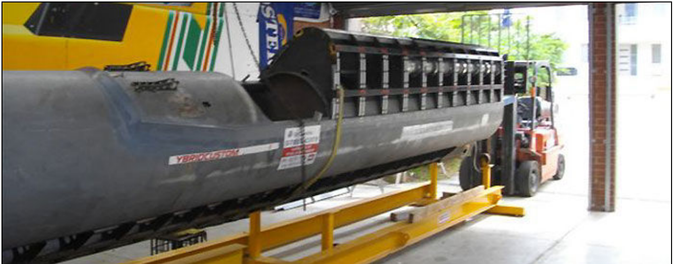
Aussie Invader 5R slowly be rotated until it is upside down for the fitting of the "V" underbelly panels
